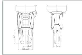
The drawing shows the optional finger set mounted on the basic version of the gripper with open jaws.
