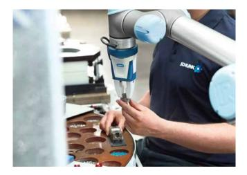
Electric 2-Finger Parallel Gripper | Small Part Gripper
