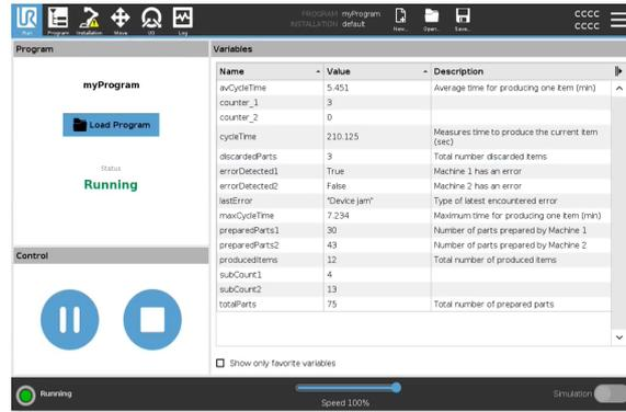
**Control** The Control pane allows you to control the running program. You can play and stop, or pause and resume a program, using the buttons listed in the table below:
