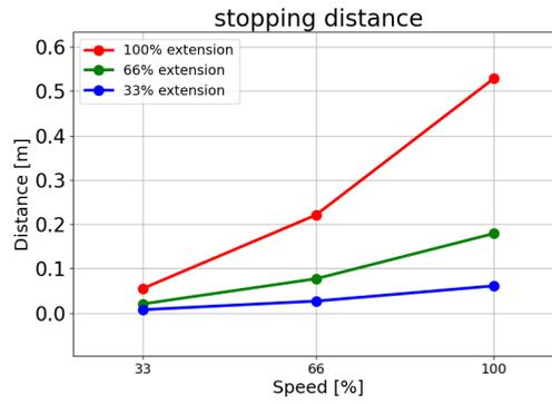
Stopping distance in meters for 66% of 17.5kg
