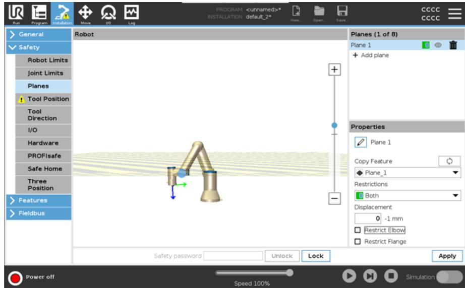
The unrestricted tool flange can cross a safety plane, even when no tool is defined. If no tool is added, a warning on the Tool Position button prompts you to correctly define the tool.
