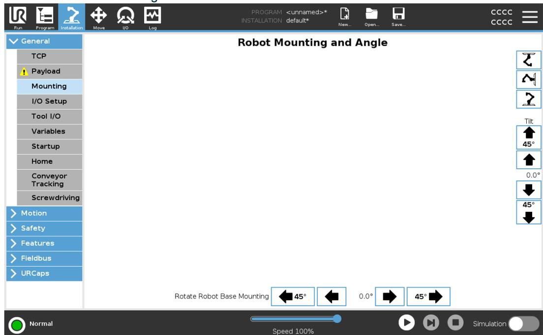
An advanced dynamics model gives the robot arm smooth and precise motions and allows the robot arm to hold itself in Freedrive. For this reason, it is important to mount the robot arm correctly.
