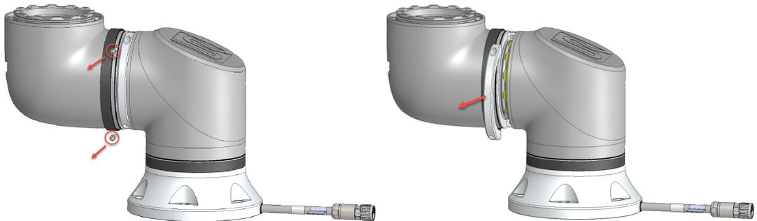
4. Support the joint as you remove the second side of the clamp.
