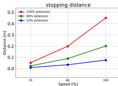
Stopping distance in meters for maximum payload of 17.5kg
