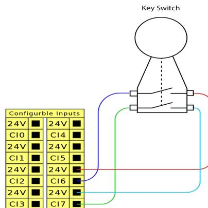
**To configure the connected safety inputs**
