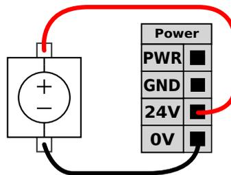
In this example the configuration uses an external power supply for more current.
