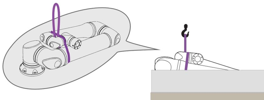
4. Lift the robot arm out of the box using the strap and hook.
