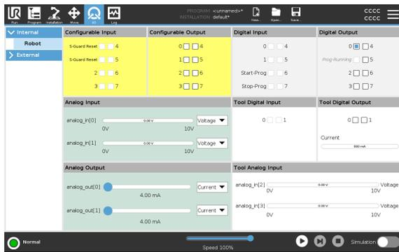
**Voltage** When the Tool Output is controlled by the user, you can configure Voltage. Selecting a URCap removes access to Voltage.
