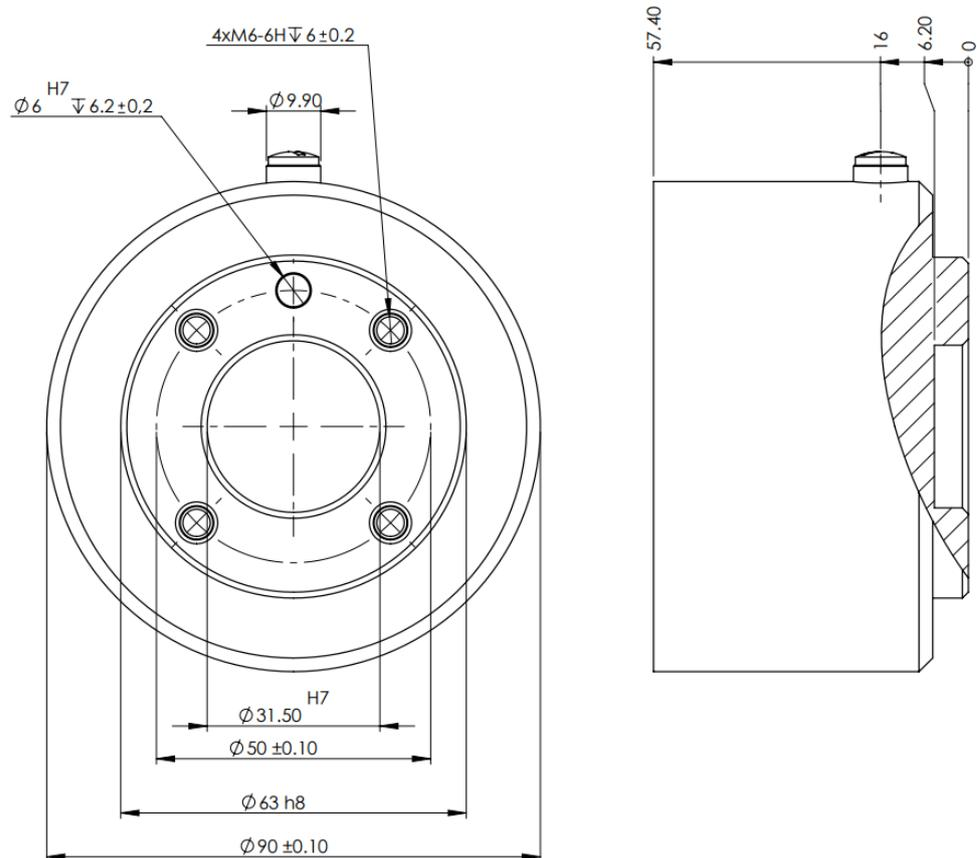
Dimensions and hole pattern of the tool flange. All measurements are in millimeters.
