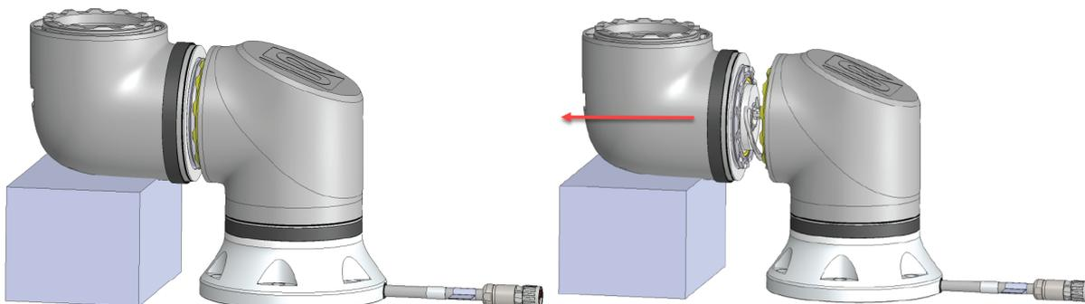
6. Gently unplug the connector from the PCB on joint.
