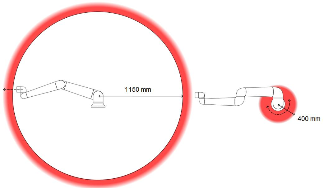
*Due to the physical properties of the robot arm, certain workspace areas require attention regarding pinching hazards. One area (left) is defined for radial motions when the wrist 1 joint is at least 1150 mm from the base of the robot. The other area (right) is within 400 mm of the base of the robot, when moving tangentially.*
