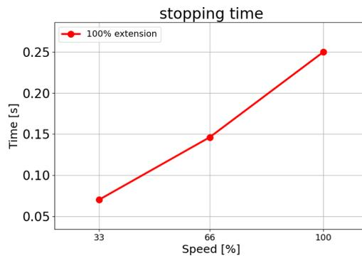
Stopping time in seconds for maximum payload of 17.5 kg
