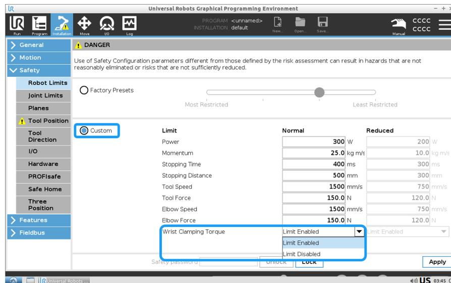
4. Tap **Apply** and **Confirm Safety Configuration** to apply the safety configuration and restart the safety system.
