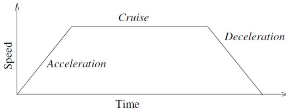
**1.1:** *Speed profile for a motion. The curve is divided into three segments: acceleration, cruise and deceleration. The level of the cruise phase is given by the speed setting of the motion, while the steepness of the acceleration and deceleration phases is given by the acceleration parameter.*
