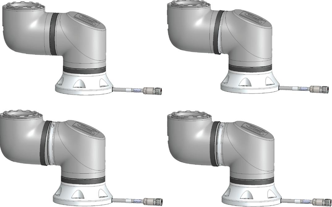
3. Remove the screws and the clamp on one side.
