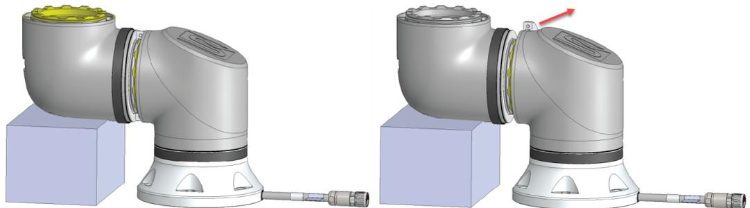
5. The joint is now loose and can be removed.
