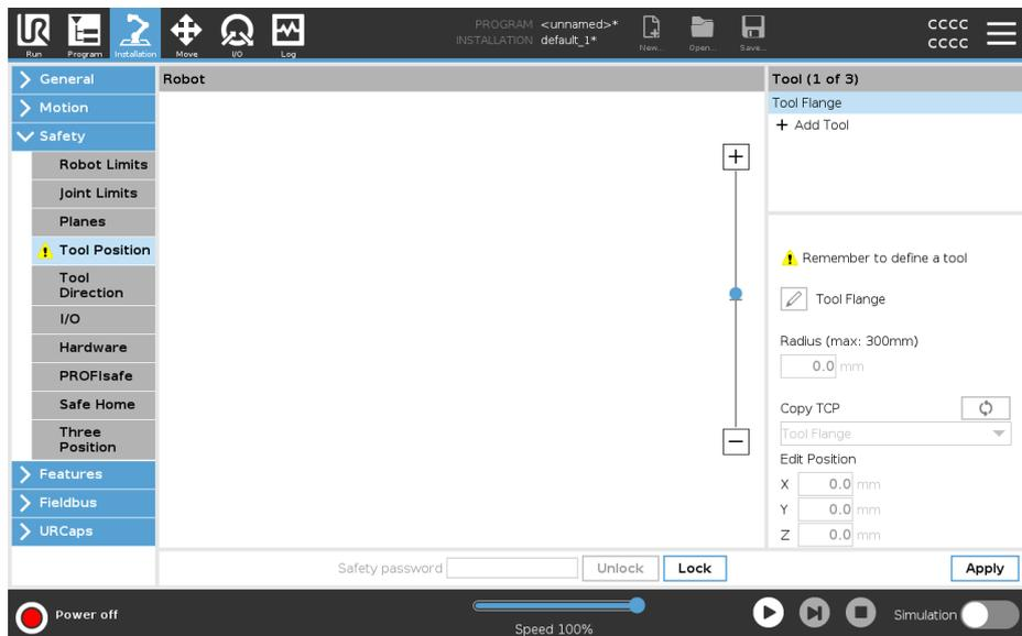
**Tool Position Warning** You must set a Tool Position within the safety settings, for the safety plane to trigger correctly when the tool TCP approaches the safety plane.
