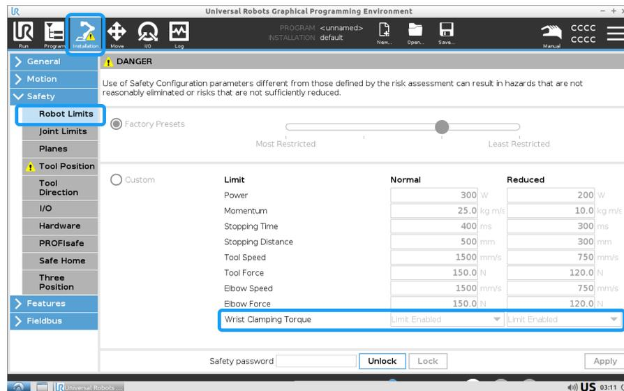
2. Under **Robot Limits**, tap **Safety password** field. Unlock, enter the safety password, and apply and restart.
