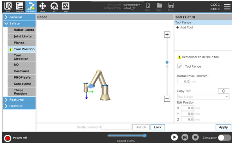
Tool Position button without the warning indicates a tool (other than the Tool Flange) is added.
