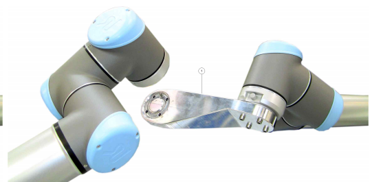
Calibration Connector attached to the Master robot's tool flange and the Slave robot's tool flange (step 5).
