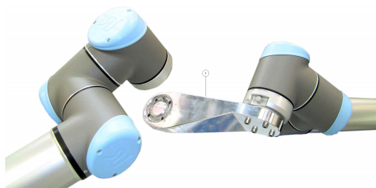
Calibration Connector attached to the Master robot's tool flange (step 2).
