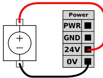
In this example the configuration uses an external power supply for more current.
