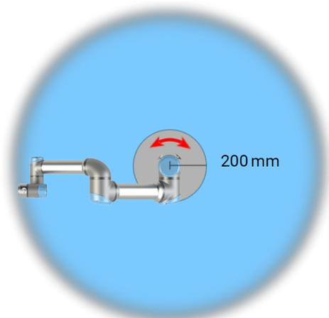
*Due to the physical properties of the robot arm, certain workspace areas require attention regarding pinching hazards. One area (left) is defined for radial motions when the wrist 1 joint is at least 750 mm from the base of the robot. The other area (right) is within 200 mm of the base of the robot, when moving tangentially.*
