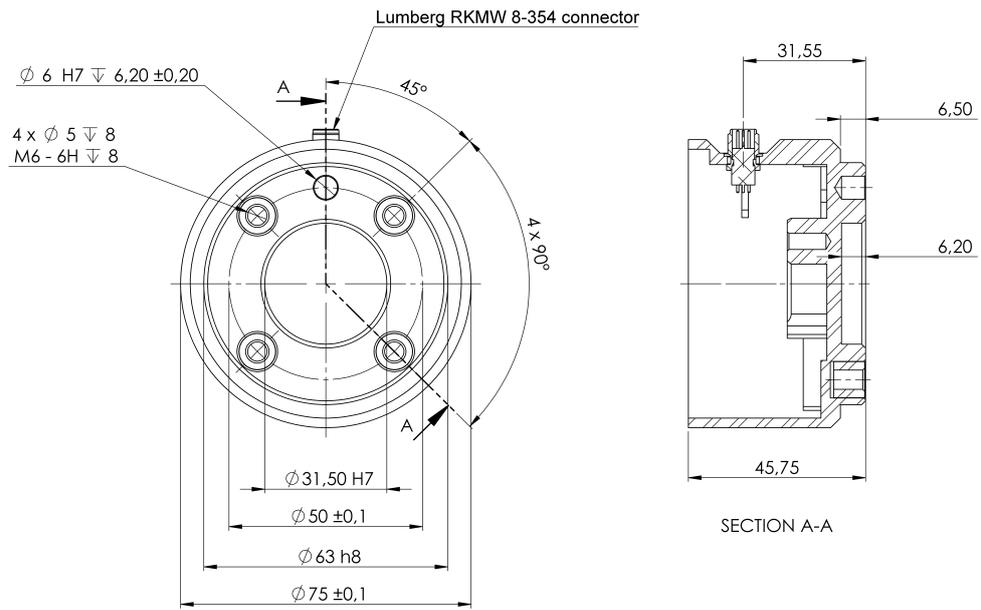
Dimensions and hole pattern of the tool flange. All measurements are in millimeters.
