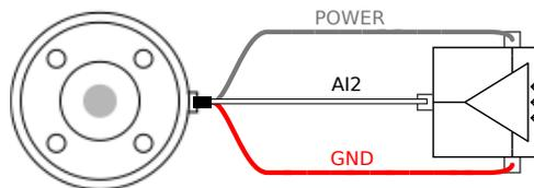
**Using Tool Analog Inputs, differential**
