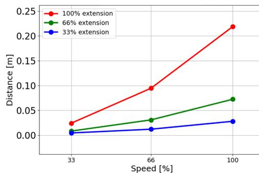
Stopping distance in meters for 66% of 7.5kg
