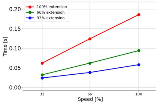
Stopping time in seconds for maximum payload of 7.5kg
