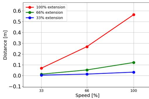
Stopping distance in meters for maximum payload of 7.5kg
