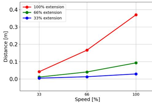
Stopping distance in meters for 66% of 7.5kg
