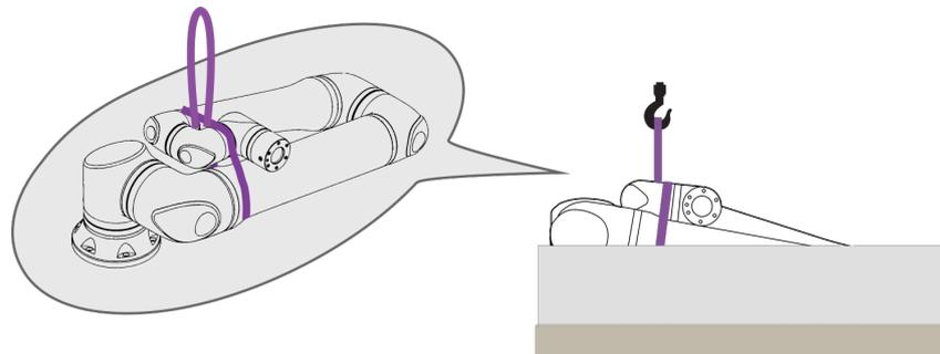
4. Lift the robot arm out of the box using the strap and hook.
