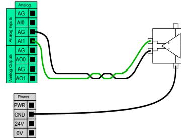
This example illustrates connecting an analog sensor.
