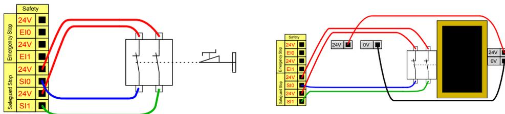
In this example a door switch is a basic safeguard device where the robot is stopped when the door is opened.
