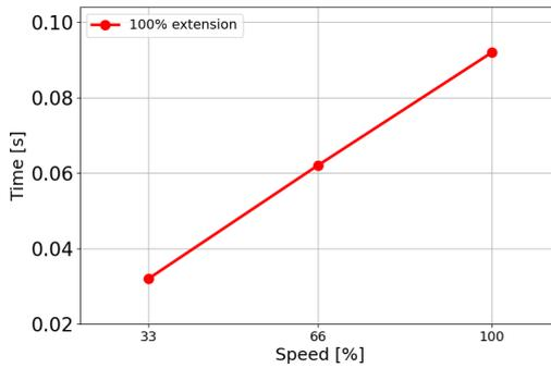
Stopping time in seconds for the maximum payload of 7.5kg
