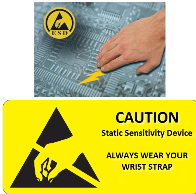
Figure 1.0 PCB, an ESD-sensitive part
