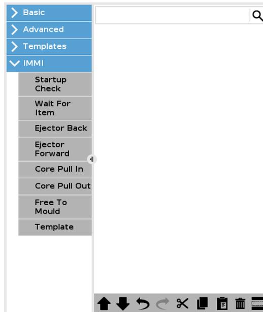
All program structure nodes consist of a set of steps. Most of the steps are enabled by default. Some steps cannot be disabled because they are essential to the program structure functionality.
