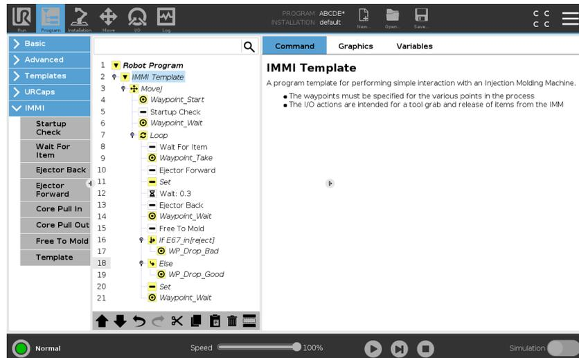
3. To prepare the robot for handling objects, select desired waypoints from the following:
