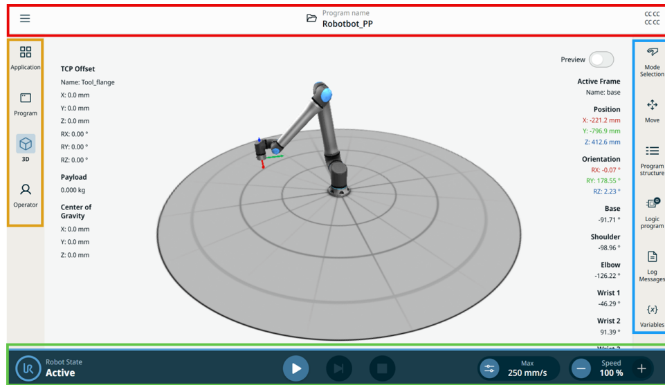
PolyScope X layout partitioned into Header, Main Navigation, Sidebar, and Footer
